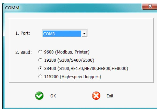
If more than one logger is connected to the PC, maybe you should choose the port manually. Don't care about the baud, if you forget it, the software will check the baud automatically.
