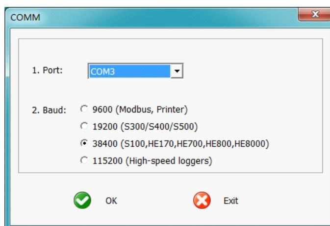
If more than one logger is connected to the PC, maybe you should choose the port manually. Don't care about the baud, if you forget it, the software will check the baud automatically.
